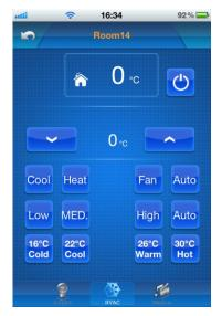
ON/Off Temperature Control Fan Speed, Low, Mid, High Mood: Heating, Cooling, Fan, Auto Presets: Cold, Cools, Warm, HOT
